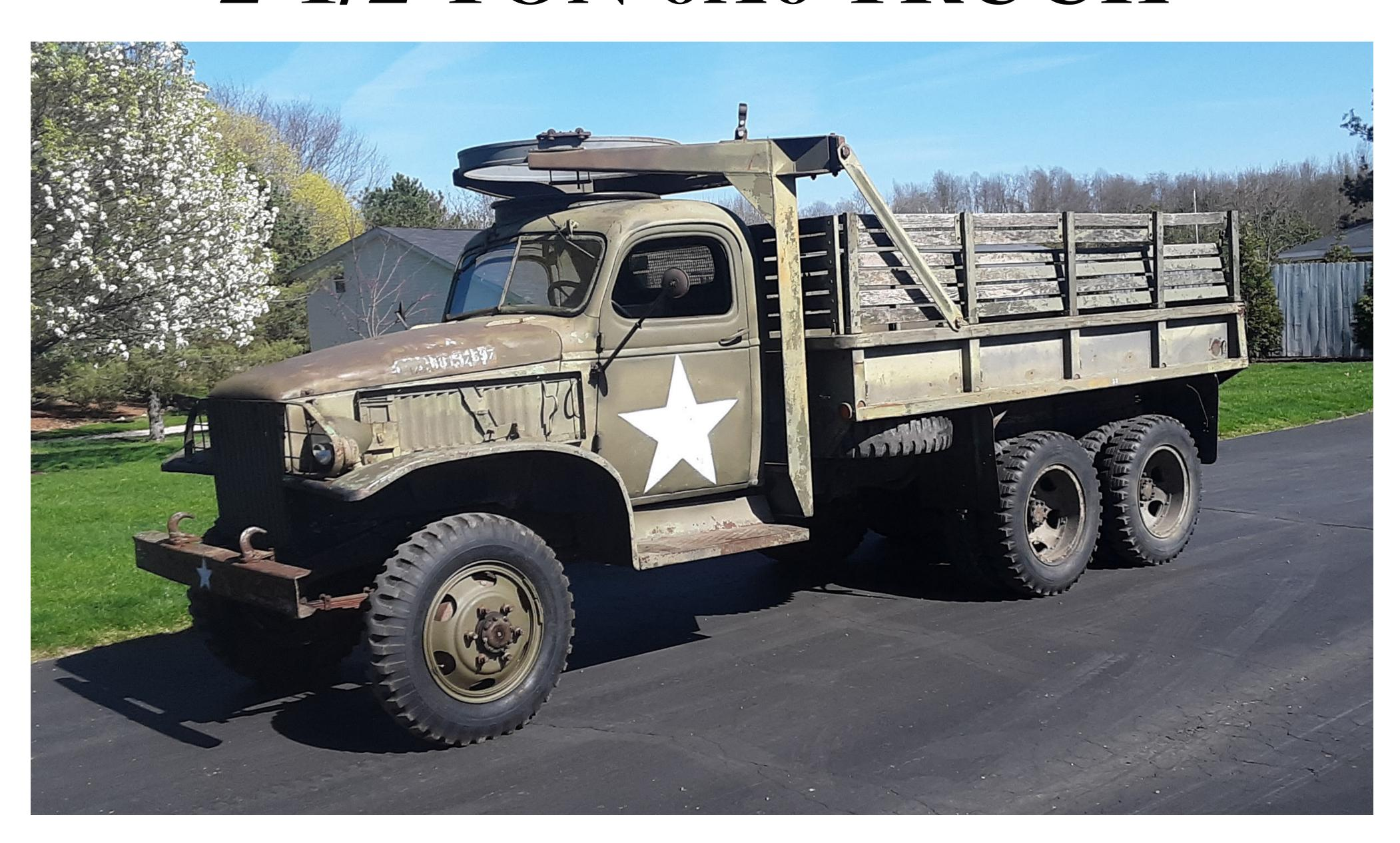
The GMC CCKW truck, also known as the "Deuce and a Half," is an iconic military vehicle that gained popularity during World War II. Produced by General Motors, the CCKW was a 2.5-ton six-wheel drive truck that played a crucial role in transporting troops, supplies, and equipment across various terrains. Its sturdy construction and off-road capabilities made it a reliable workhorse on the battlefield.
